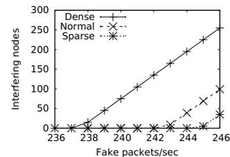
Figure 2: Interfering nodes in relation with the number of fake packets/sec.
