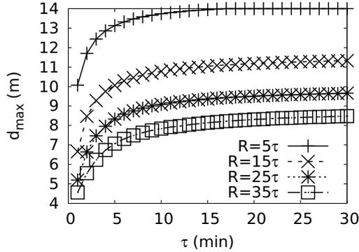
Figure 2: Maximum drone distance  $d_{max}$  for different packet intervals  $\tau$  and maintenance starting times  $R\tau$ .
