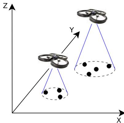
Figure 1: Two drone positions with different altitude charging a number of nodes.
