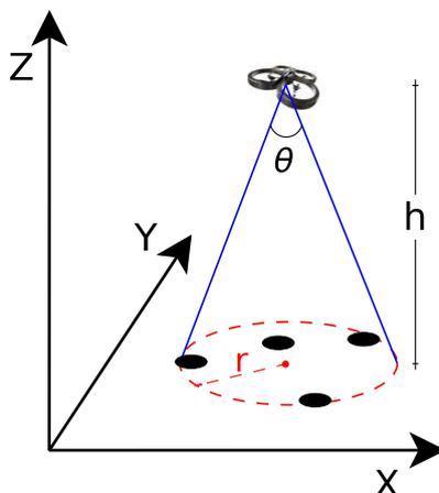
Figure 3: A drone with altitude  $h$  and covering radius  $r$ .
