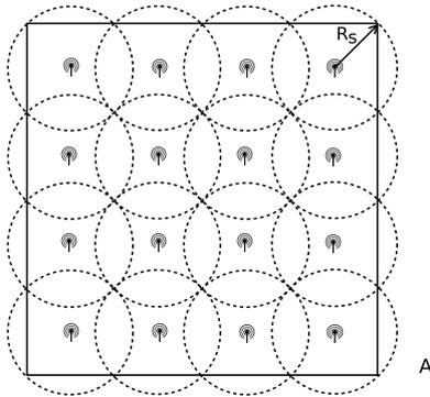
Figure 2: The maximum square area covered by 16 nodes using the quadratic node deployment.
