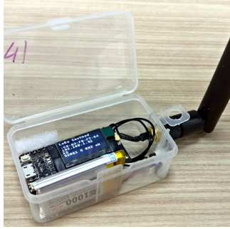
Figure 10: Custom built of a TTGO SX1276 LoRa end-device.
