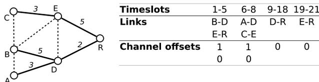
Figure 1: Example topology and the corresponding LOST scheduling.
