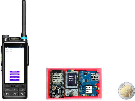
Figure 5: A TETRA terminal (left) equipped with Android software to communicate with a station device (center), and size comparison with a 2€ coin (right).
