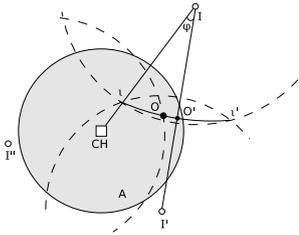
Figure 1: Example with the positions of three distant nodes, the intermediate charger positions and the optimal position on the plane.
